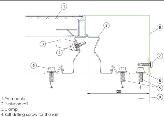
5.Self drilling screw for the purlin
