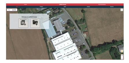
Fill in the fields and enter the address of the project. AdiWatt-Design works with Google Maps, this will allow you to work on the right roof. In case your project is located in hurricane zone, select «hurricane zone», this will induce the addition of material for the supply list. Validate and start working.
